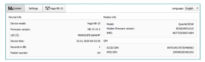
**Device info** - the configurator reads information about the device model, its firmware and automatically corrects the device's time when connected to it. In that block you can find out the number of records in the black box and the number of packets sent by the device.
