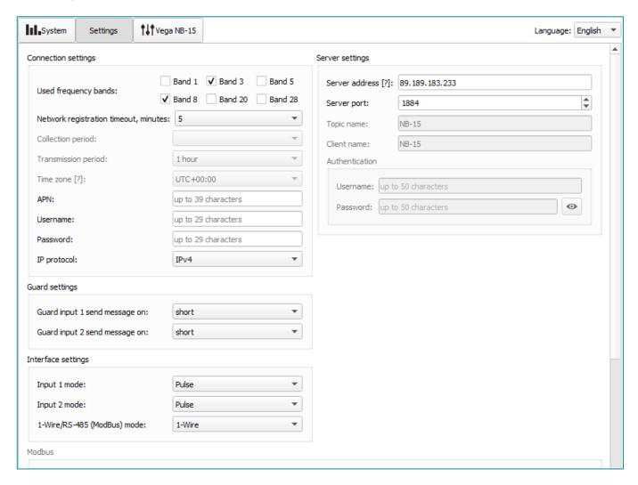
**Connection settings** – a group of parameters set up the data collection and transmitting.
