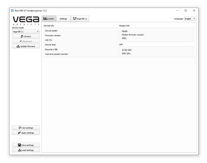
The menu on the left allows you to select the device model, connect to the device or disconnect from it, and update firmware.
