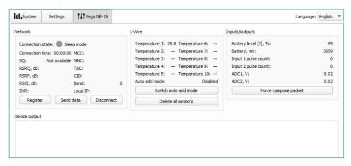
**Network** – displays the current parameters of the connection and allows to control it. Buttons in this block have logic like INIT button on the board.
