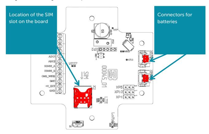
Vega NB-15 modem can be powered from either an external power source or built-in battery. To operate from the built-in battery, you must connect the battery connector to the one of power connectors on the board which XP7 or XP6 marked. In case of operation with two batteries you should use the both connectors.
